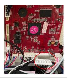
Pull out the wire and plug the wafer
