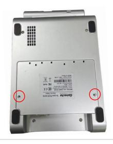
Turn the printer upside down, remove the two screws located on the bottom cover, and open the bottom cover.
