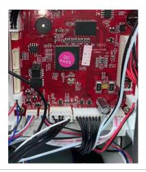
7. After inserting it, cover the bottom cover and lock the screws.
